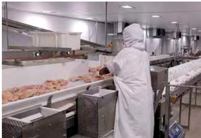
In Scanvaegt's largest IQF poultry processing solution in South Africa, the frozen meat is conveyed to the three auto-weighing and batching systems. Shown here is the product-identification carousel. These new lines complement the existing four single and two twin-processing lines for grading and batching IQF products.
