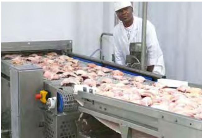
In the early 1980s, County Fair was the first company in South Africa to install a spiral freezing system for IQF processing. Pictured here is the infeed section of the new Jackstone spiral freezer.
